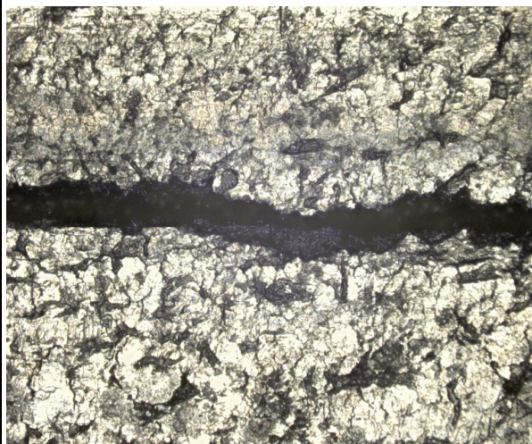
fig(3) 開裂外觀_100X
